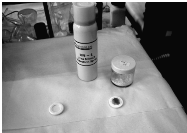
FIG. 5—UN-1 color test for traces of urea nitrate (7). Left button: negative, and right button: positive response.
