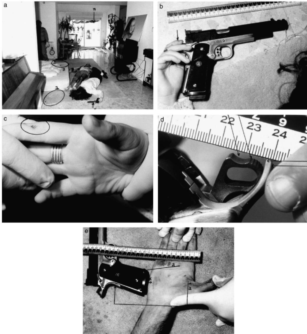
FIG. 11—Resolving a suicide-homicide case by Ferrotrace (25): (A) overview of the crime scene, (B) weapon as found adjacent to girl's right hand, (C) Ferrotrace mark on girl's index finger caused by contact with gun's hammer after death, (D) upper back of gun's hammer, which caused the Ferrotrace stain, (E) Ferrotrace stain on male victim's right hand. (Courtesy: Mobile Laboratory for Serious Crime Scenes, DIFS.)
