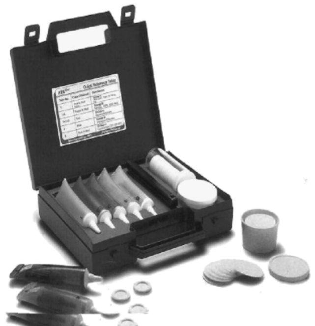
FIG. 2—Explosives Testing Kit (ETK). Each one of the colored tubes detects a different family of explosives.
