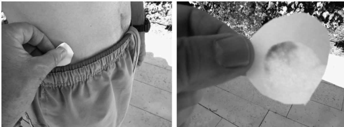
FIG. 3—Explosive Testing Kit testing for explosives traces on suspect's stomach. Left: sampling and right: positive response for nitrate and nitramine-type explosives.
