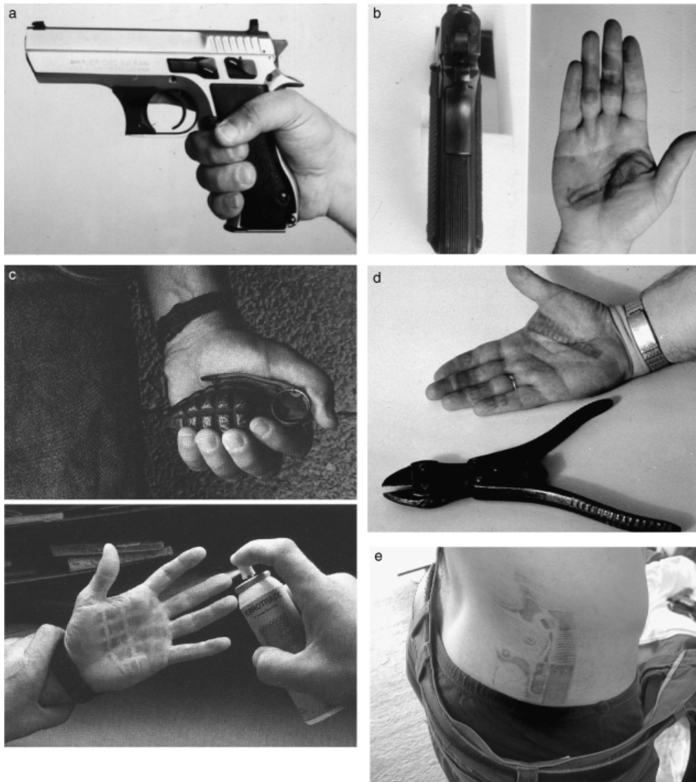
FIG. 10—Detecting recent contact with firearms by Ferrotrace: (A) by holding a gun firmly, microscopic amounts of iron are transferred to the hand, (B) Ferrotrace mark developed on hand after holding a Colt 45' pistol, (C) hand grenade mark, (D) Ferrotrace mark after holding a cutter, (E) Ferrotrace mark after carrying a pistol on the hip.
