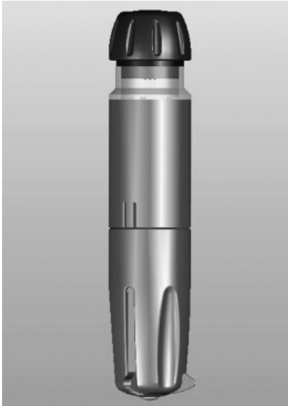
FIG. 8—Keinan's PET for detection of peroxide explosives (15).
